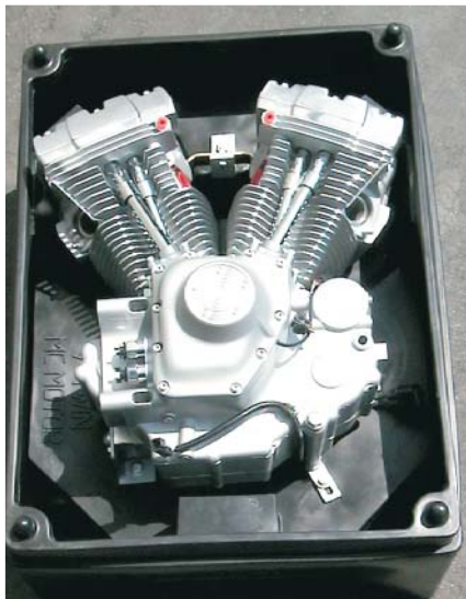
Engine bolted to container insert. 2000 engine shown requires bracket modification.
